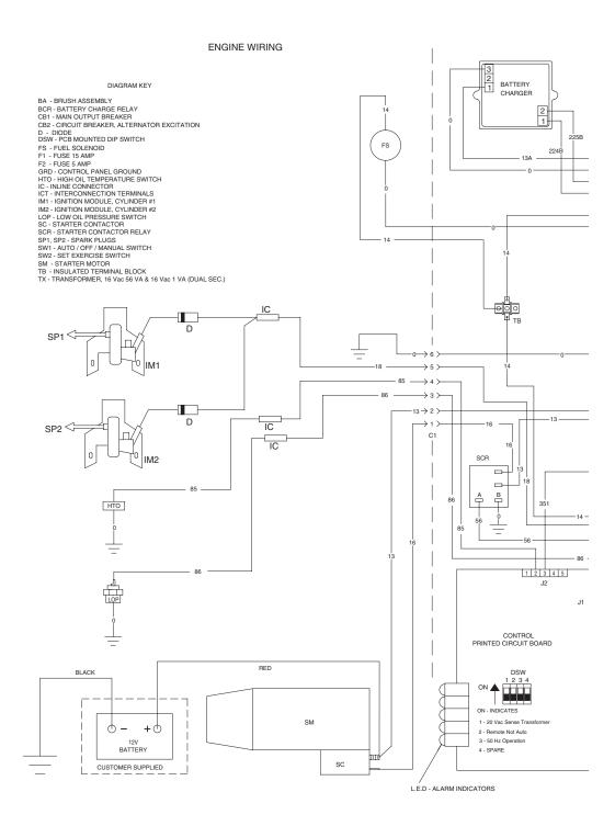
Air-cooled 8.5 kW Generator Wiring Diagram - 8.5 kW - Drawing No. 0D8500
